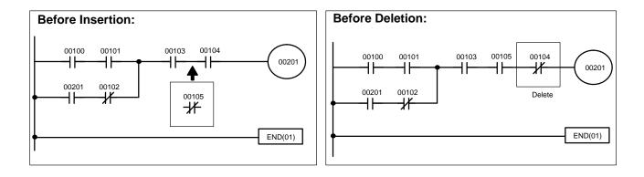
The following key inputs and displays show the procedure for achieving the program changes shown above.
